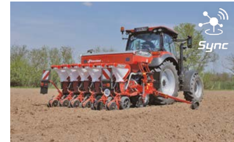
Kverneland Optima R Light rigid frames from 3.0 to 6.0m for different row types like standard, tandem, HD-II and SX rows.
