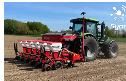
Kverneland Optima V The variable telescopic frame for various crops and row widths (33 to 80cm) for farmers and contractors. With HD-II or SX row.
