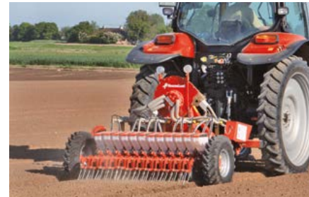
Kverneland Miniair Nova (vegetable) For all sorts of vegetable seeds. Made to ensure highly accurate seed placement.
