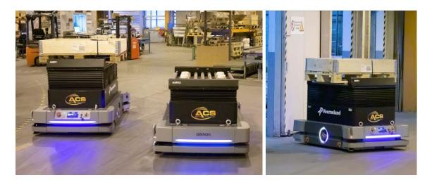
AGV robots produced by Omron, working autonomously in the warehouse, improving safety and increasing efficiency and productivity
