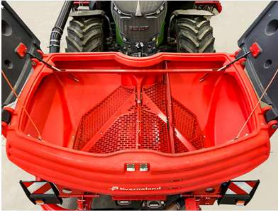
Kverneland fronttank f-drill maxi plus, tanksplit 60:40
