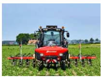
Kverneland-Onyx inter-row cultivator in combination with iXtra LiFe for band spraying in combined operation (image 3)
