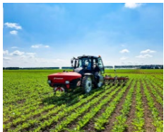
Kverneland-Onyx-inter-row cultivator in combination with iXtra LiFe for band spraying in combined operation (image 2)
