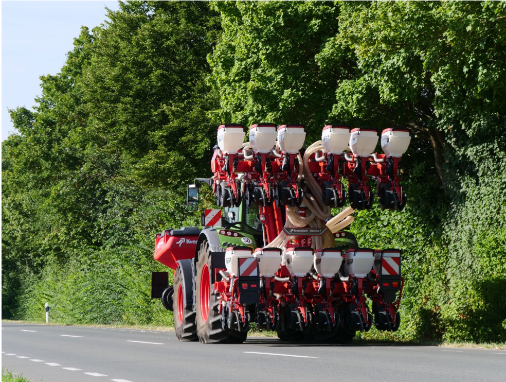
Quickly fold to transport position: Optima F with 12 SX units
