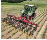
Kverneland-inter-row cultivator Onyx with Lynx guiding interface in maize field (image 1)
