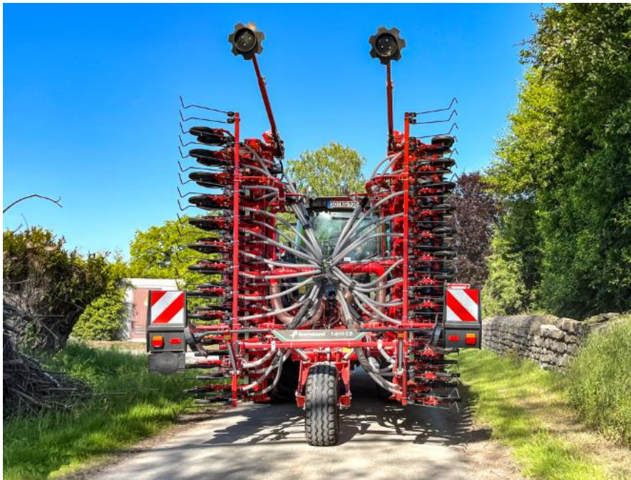
Kverneland coulter bar f-drill CB F safe road transport with support wheel
