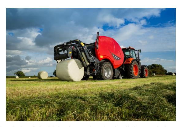
Kverneland unveils FastBale Premium, an enhanced version of its famous and unique non-stop baling breakthrough baler- wrapper combination. It features higher cost-effectiveness in operation, easier-to-use solutions and an improved reworked chopping system with increased capacity and easy access to knives.
