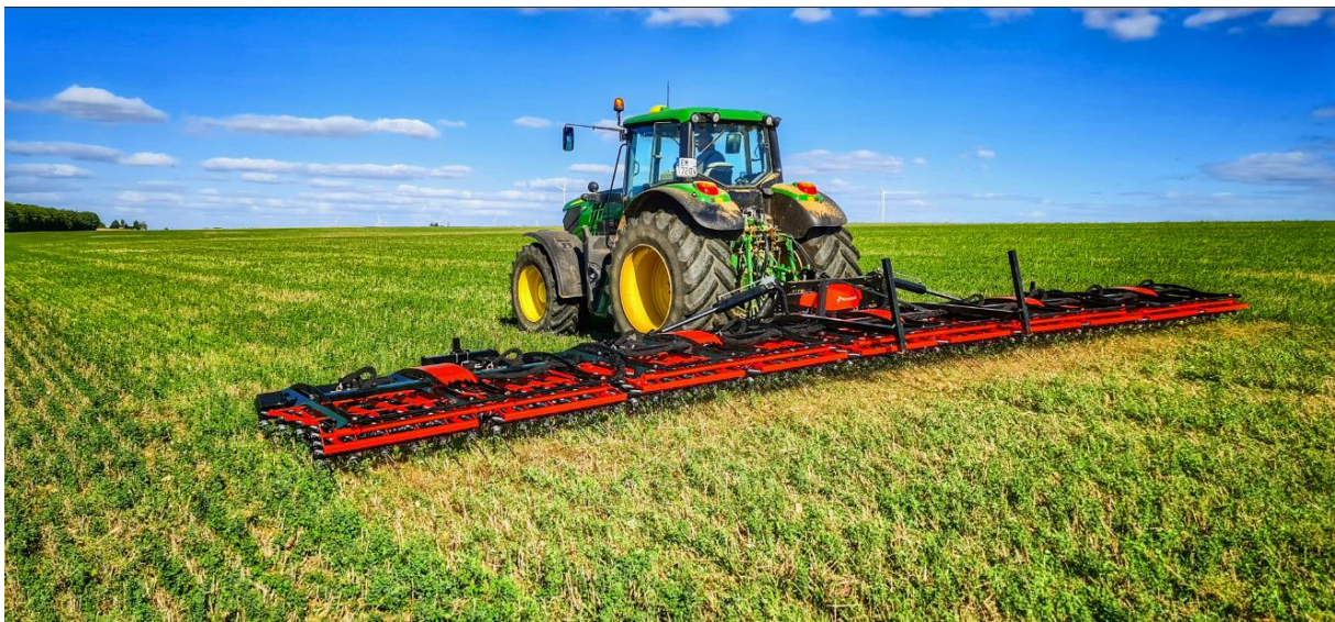
Kverneland Arcadia tine harrow with 12m working width
