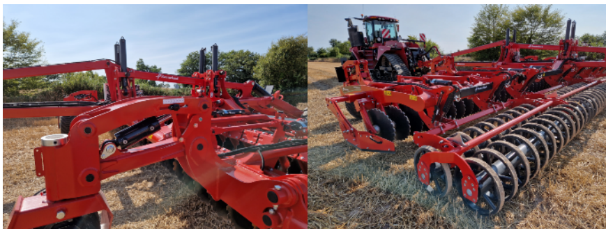
Kverneland Qualidisc 21123 T pre-setting of the depth at the front and rear of the machine
