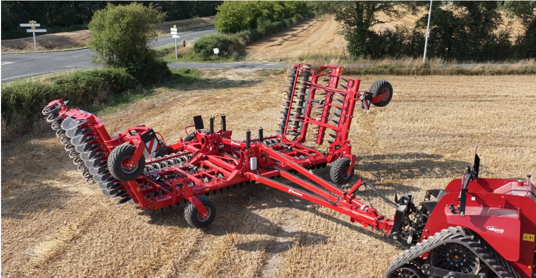
Kverneland Qualidisc T is folding as wallet system
