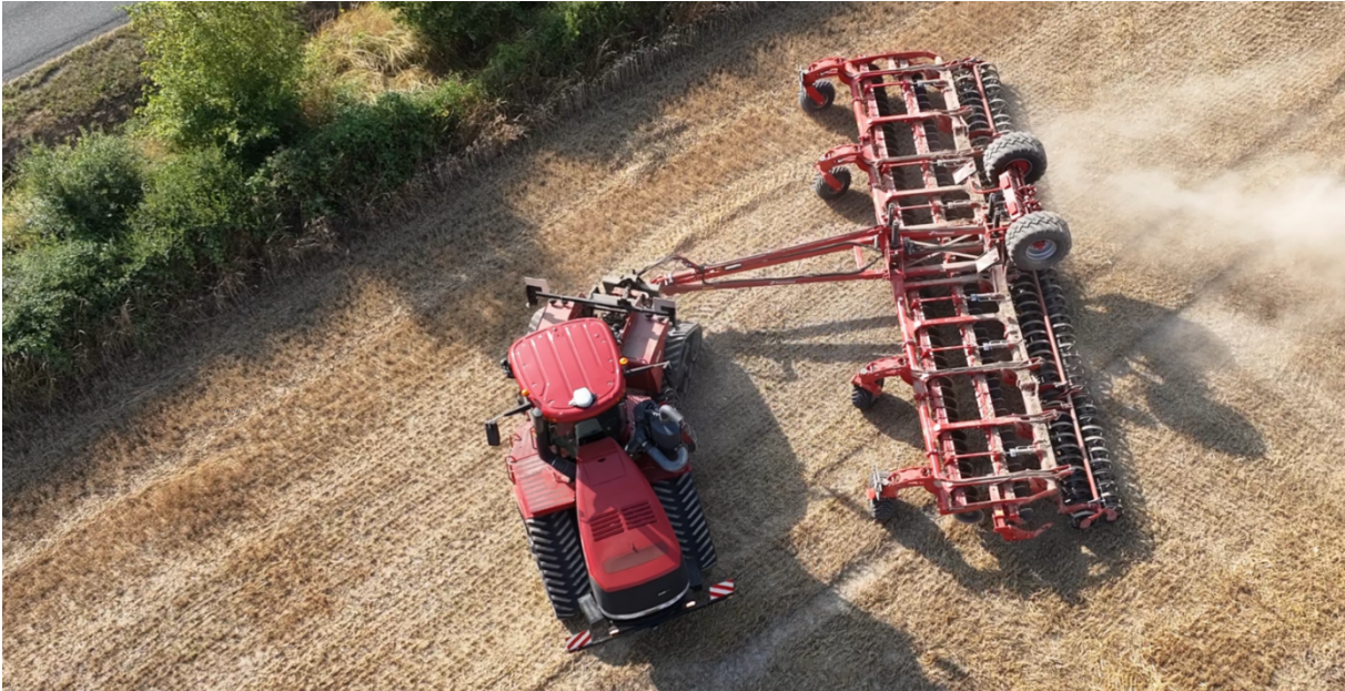
Kverneland Qualidisc T headland turn on gauge wheels and rear roller
