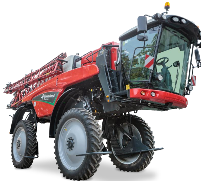
iXflex hydraulic ground clearance adjustment for Kverneland iXdrive S6
