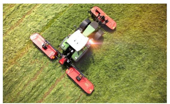
The Vicon EXTRA 495 plain mower without conditioner offers significant mower capacity with its 9.5m working width and QuattroLink suspension concept.
