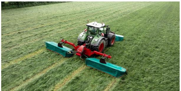
The new Kverneland 5395 plain triple mower featuring 9.5m working width and the innovative QuattroLink suspension system, delivers impressive mowing capacity.
