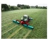
Kverneland 5395 plain triple mower with 9.5m working width
