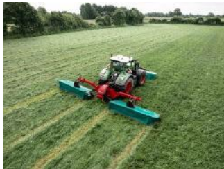
Kverneland 5395 plain triple mower with 9.5m working width
