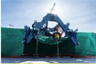
[Direct tractor coupling without the need of an A-frame](#)
