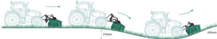
[The mowing unit has an adaptation range of 430mm upwards and 210mm downwards](#)
