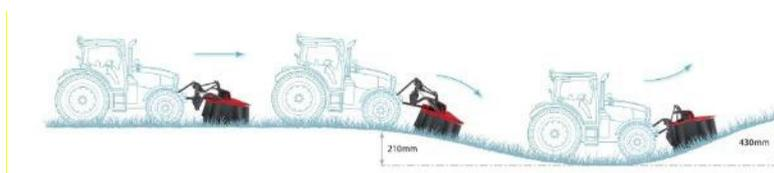
[The mowing unit has an adaptation range of 430mm upwards and 210mm downwards](#)
