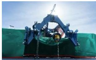
[Direct tractor coupling without the need of an A-frame](#)
