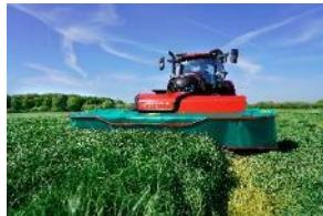
[Kverneland 2800 F series is available in 2.8, 3.2 and 3.6m working widths](#)
