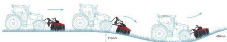
[The mowing unit has an adaptation range of 430mm upwards and 210mm downwards](#)
