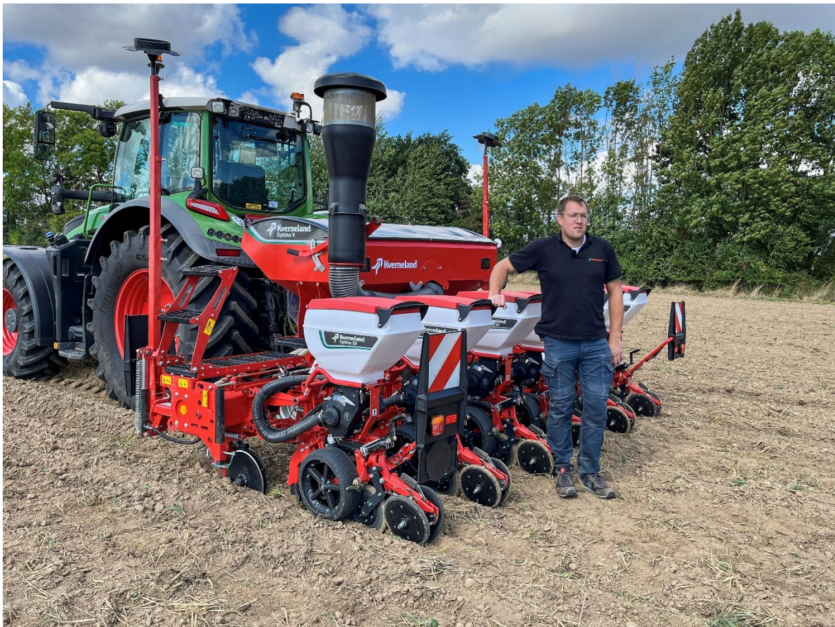
Kverneland Optima V SX sowing row with GEOFORCE system
