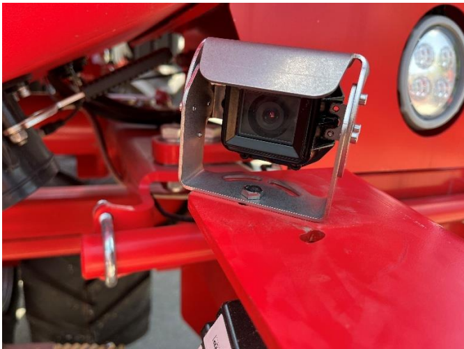
New front camera system improves visibility and safety
