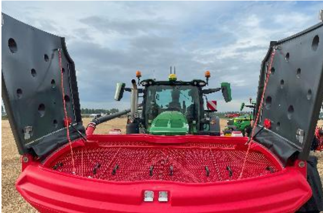
Easy access to the hopper – new sieve design increases operator's convenience
