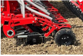
Kverneland CX-II without press wheel
