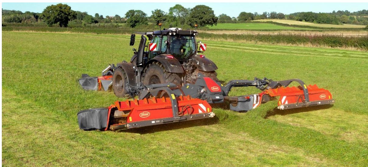
The new Vicon EXTRA 7110 triple mower combination with 10.2m working width and the new innovative CurvePilot solution.
